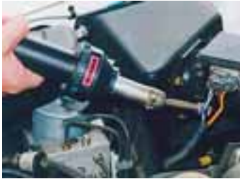
HOT JET S with spoon sieve reflector for solder shrinking.
